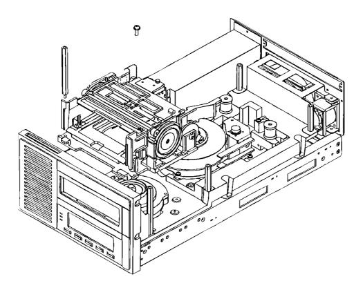
Figure 8-10. Loader Assembly
